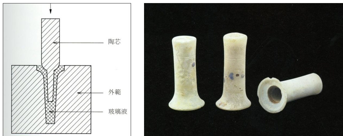
Fig. 4: Left, a diagram of a double-mold used to make ear studs. Clay residue in the hollow areas of these ear studs suggest that after annealing, the outer mold was broken off while the inner mold was melted with water. Right, the resulting hollow glass ear studs. Source: (Kwon 2001:53, 225).
